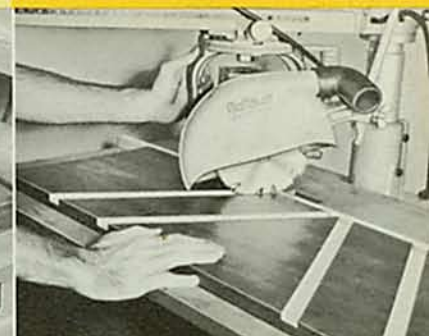
PARALLEL LEFT HAND DADO. Swivel the motor 180°, swing arm left to desired angle. Mark your guide fence and make successive cuts the exact distance apart.
