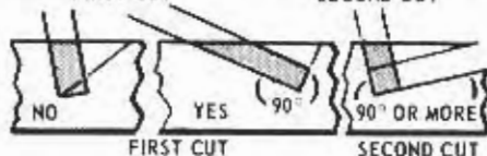
V-GROOVES IN TWO CUTS
