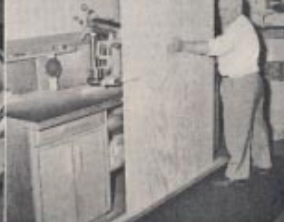
HORIZONTAL SAWING. Tilt motor vertical, set saw parallel to table top and cut across 4 foot wide panels this way. Saw can be lowered or raised for desired width.
