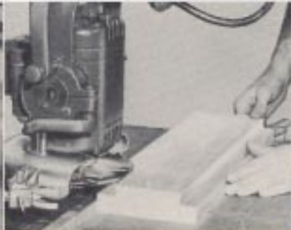
RABBIT-CUT. By taking advantage of the dado diameter, you can make wide-width rabbet cuts with amazing ease and speed!
