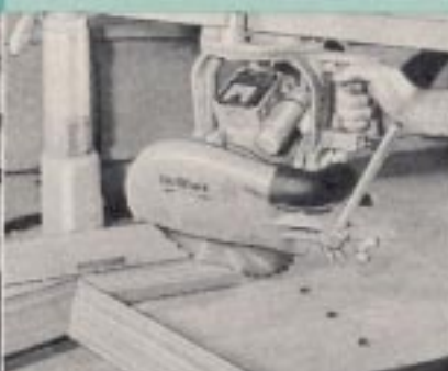
SHADOW BOX CUT. Set arm at 30° R. H. miter, tilt saw 35° PLUS on bevel . . . then duplicate cuts for each end, positioning stock as needed.
