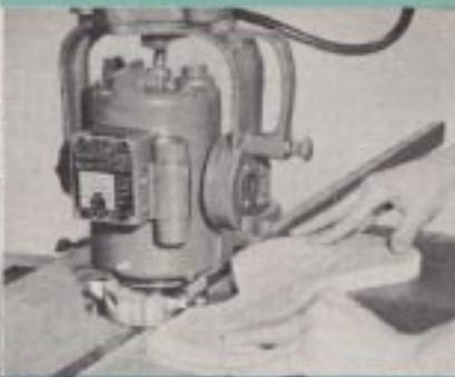
IRREGULAR SHAPING. Made easy with the use of a shaper ring to guide the stock. Remove the guide fence and work the irregular stock past the cutter for moulding.
