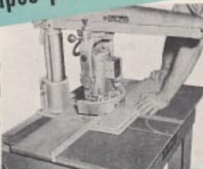
BEAD AND COVE CUT. Push the shaper cutter in or out . . . raise or lower . . . or tilt to any angle and you quickly multiply the number of different shapes from a single cutter. Exclusive Shaper Guard Protects You.
