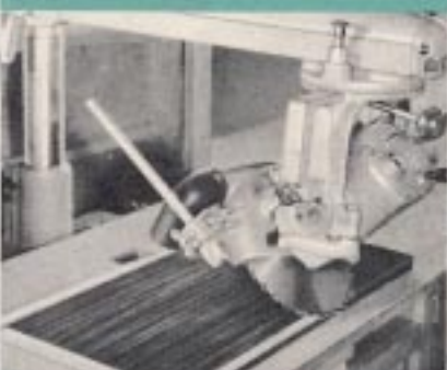
CHAMFER CUT. Easy way to make bevel cut along four top edges of stock . . . or cut "V" pieces for cylindrical patterns.
