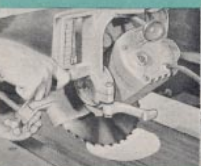
SAUCER CUT. Clamp stock to table, arc swing and lower saw blade until desired depth is reached. Makes intricate decorative patterns easily.
