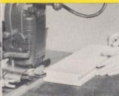
GROOVING. Dado Head gives you extra-wide groove cuts, eliminating a number of passes when made with saw blade alone.
