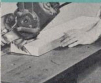
BEVEL-RIP. Involved in making modern-type drawer pulls, chamfer strips, and cylindrical pattern work.
