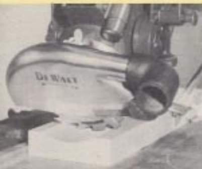
RADIUS CUTTING. Tilt dado, and push work through as in ripping—and you get a fine concave cut full length of the board.
