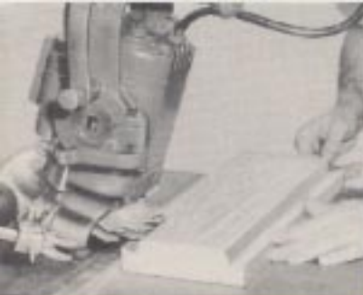
BEVEL RABBIT-CUT. Simply tilt the motor and you can make any desired angle cut in your rabbeting operation.
