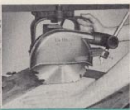
RIGHT-HAND MITER CUT. Simply set the arm at the desired angle and the problem of picture frames, boxes, etc., is solved! One motion does it!
