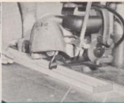
2-POINT SOLID MOULDING CUTTER. Makes decorative patterns on the edge, side or above the material simply by adjusting the AMF DE WALT cutter head where desired. Note the safety guard covering.
