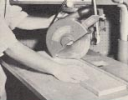
LEFT-HAND MITER. By turning saw 180° to opposite side, difficult left-hand miters are accomplished in the middle of the work table—easily, perfectly.
