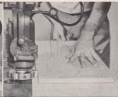
SIZING AND JOINTING. Put guide fence at front of regular table, position the cutter for width desired. Every board that passes through is perfectly sized and jointed.
