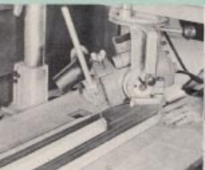
CONTOUR CUTTING. Simply tilt and swivel the motor to use saw kerf for the contour you want the full length of the board.
