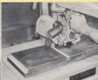
CUT OFF AND DADO. Saw blade and dado head combine to give you this unusually fast, accurate job in a single operation.
