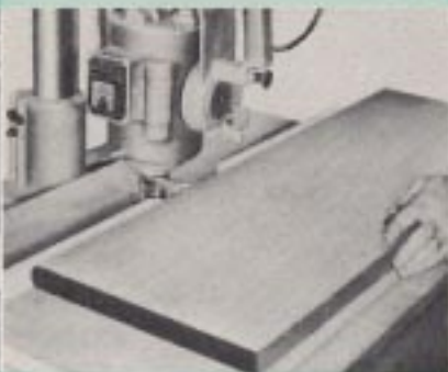
MAKING STAIR TREADS. A full sized nosing cutter puts the half-round shape along the edge of the stair tread . . . a highly important millwork operation done at home.
