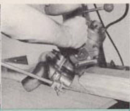
BEVEL MITER. Combining the two operations of mitering and beveling is a simple matter. Set the arm, angle the saw, and move the saw across your work!
