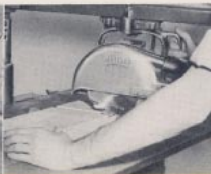
ANGLE DADO. A special cut which finds many uses, accomplished similar to mitering with saw!
