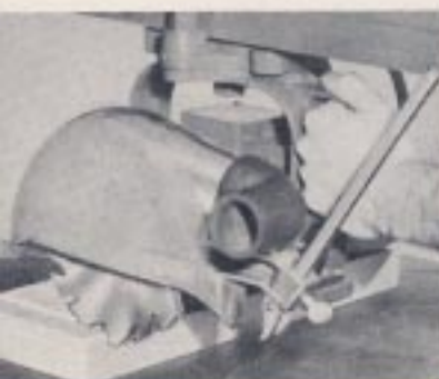
CROSS DADO. For fitting ends of shelves into sides of bookcases—and countless other uses!
