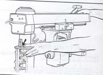
Remove Column Support trim using screwdriver as shown.
