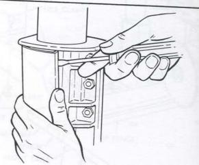
3. Loosen (2)  $\frac{1}{4}$  – 20 Gib set screws on the left side at the rear of the column support.
