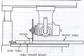
e. Position carriage until the edge of the blade, when spun by hand, just touches the front face of the fence. The rip-scale indicator (on the right hand side of radial arm) should now read "0" inches on upper portion of the blade "In-Rip" scale. If not, loosen screws and shift the indicator until it is aligned with the "0" mark, then tighten the screws.
