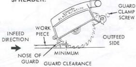
The blade guard is positioned by loosening the guard clamp screw and rotating the guard so that the nose just clears the workpiece as shown.
