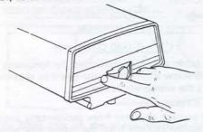
c. Push lever in - with thumb - to turn switch off.
