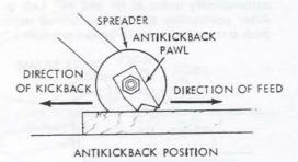
Loosen the wing screw and with the tab provided, position the antikickback and spreader assembly until the pawl assumes approximately the position shown above. Tighten the wing screw.
