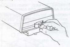
Insert finger under end of switch lever and pull end out, to turn switch on.
