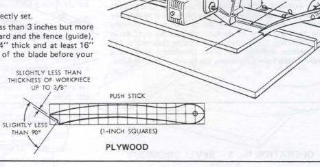
When ripping stock 1/4 inch or less between the blade and fence (guide) use a Pusher Board.
