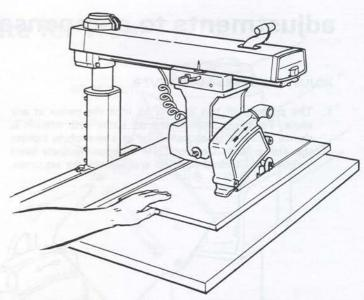
Out-Ripping. The radial arm and bevel are indexed at 0° and locked, but the yoke is turned 90-degrees in a counterclockwise direction (viewed from above), from the crosscut position. When standing in front of the saw, blade would be rotating clockwise. After positioning the guard and antikickback mechanism the workpiece is fed from the left-hand side of the saw. The "Blade Out-Rip" scale is on the left hand side of radial arm.
