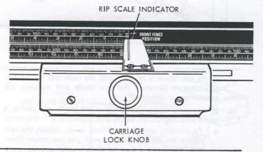
f. The blade "Out-Rip" scale indicator on the left hand side of the radial arm is adjusted in essentially the same manner as the blade "In-Rip" indicator, except the blade should be as shown. With 2 inches measured between the fence and the face of saw blade, the rip-scale indicator should be positioned to read 2 inches on the upper portion of the blade "Out-Rip" scale.
